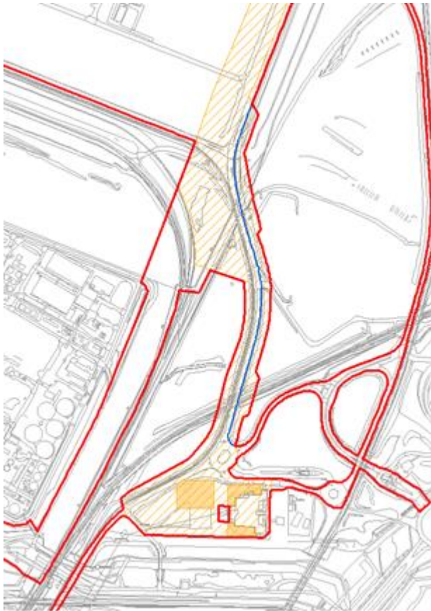
Figure 4 (Change 4) – showing approximate additional areas for inclusion into Work No. 3A (HV cabling) blue line shows existing Order Limits.
